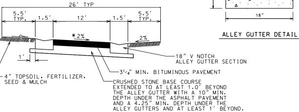
\* SEE ARROWS ON PLAN PAVEMENT FOR DIRECTION OF CROSS SLOPE.
